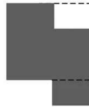
SURFACE AREA +10% Loses 10% more heat & costs +10% to build
